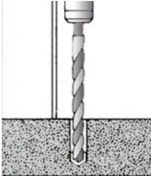
5. Before proceeding with installation, the hole must be cleaned of all concrete dust to ensure proper fastening. Use a wire brush, a vacuum or compressed air to clean out the hole completely.
