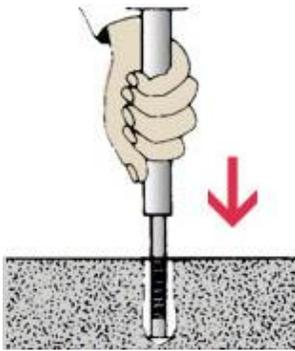
8. For the Public Work Stand - place the stand over the 4 anchors. You will be using 2 studs for the Penta nuts and 2 button head hex bolts (opposite sides from each other). You will thread the studs into the anchors prior to installing the Penta nuts using the Penta socket. Use the hex wrench to tighten the button head hex bolts.
